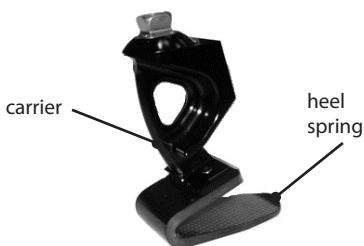
Assemble heel spring onto carrier, use Loctite 243 (926012) and torque to 15Nm. Use special Allen wrench 940080, Torque spanner adaptor 940081 or 13A/F spanner 940273.
