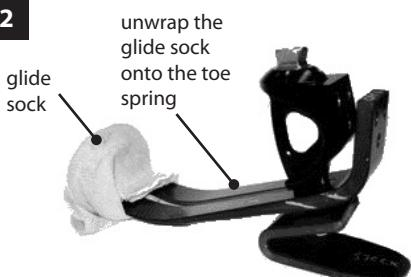
Slide toe spring into position on carrier (do not assemble bolts). Fold the glide sock neatly around the end of the toe
