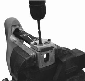
Drill two 8.1 diameter holes through drill bushes.
