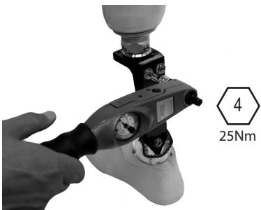
Cut blade using method shown previously before attaching top housing. Loctite (243) & tighten bolts (25Nm). Re-apply cosmesis if applicable.
