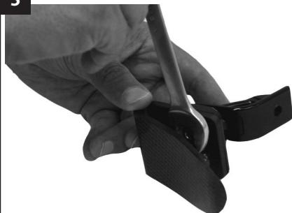
Remove heel spring from carrier.
