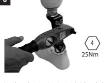
Attach top housing. Loctite 243 & tighten bolts 25Nm. Re-apply cosmesis if applicable.
