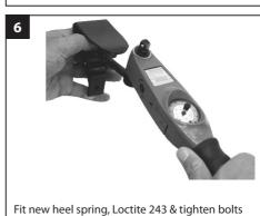
(15Nm). Use torque spanner attachment 940081)
