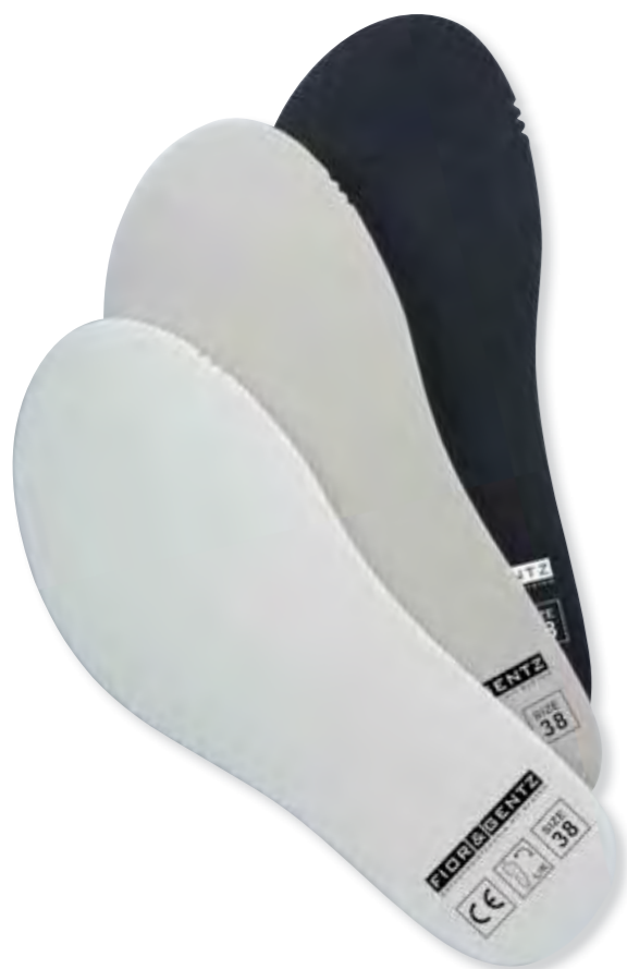
The insoles are made of EVA material and provide a different shore hardness: black = 40°, grey = 25°, white = 50°
