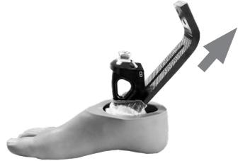
Remove securing screws from the carrier and pull the toe spring towards the rear of the foot.
