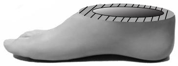
If a foam cosmesis is to be fitted, roughen top surface of foot shell to provide ideal bonding surface.
