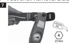
Attach blade to heel carrier. Loctite (243) & tighten bolt (25 Nm).
