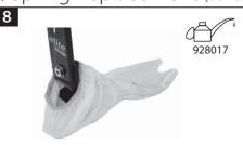
Fit glide sock and lubricate foot shell with 928017.
