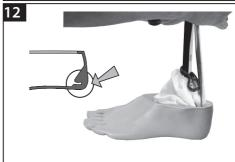
Ensure heel spring is engaged into slot.
