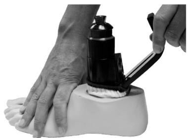
Withdraw toe spring from shell.
