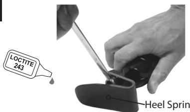
Undo and remove heel spring screws. Assemble new heel spring onto carrier, use Loctite 243 (926012) and torque to 15 Nm. Use special Allen wrench 940080, Torque spanner adaptor 940081 or 13A/F spanner 940273
