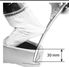
The shoe horn should be located approx. 30 mm below top surface of foot shell to ensure full engagement of heel spring.
