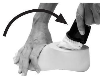
Rotate the carrier/heel spring assembly toward the rear of the foot to dis-engage the spring from its location in the shell.
