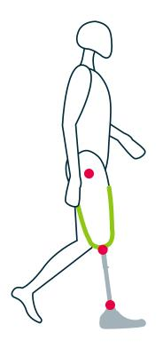
In addition to the ankle, knee and hip, the residuum-socket interface acts as an extra lower limb joint
