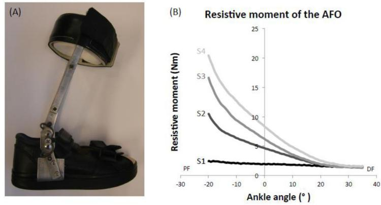
**Figure 1.** (A) The articulated ankle-foot orthosis (AFO) used in this study, (B) Plantarflexion resistance characteristics of the AFO under 4 spring conditions (S1, S2, S3 and S4) (Kobayashi et al., 2015).
