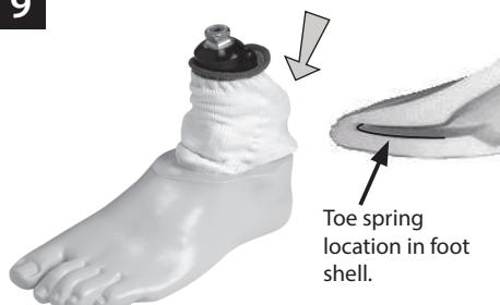
Slide carrier/heel spring assembly into the foot shell.
