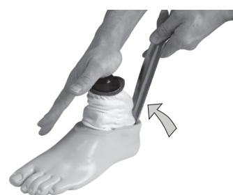
Use a suitable lever to encourage the heel spring into location in the foot shell.
