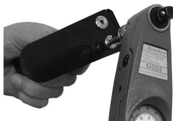
Assemble replacement heel spring, applying Loctite 243 to screw threads and torque to 15 Nm.
