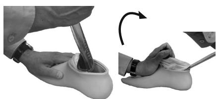
Rotate heel/carrier assembly from foot shell/glide sock.
