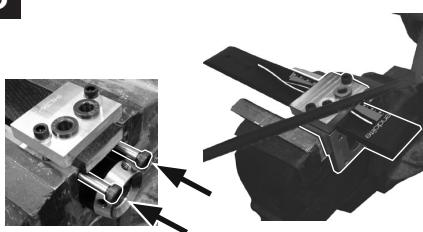
Remove socket, place fitting clamp in the vice and cut blade to length. Fit shoulder screws to prevent damage to components
