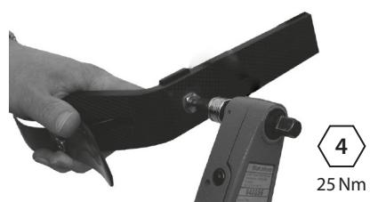
Attach pylon to carrier. Loctite (243) & tighten bolt (25 Nm).
