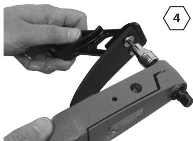
Remove heel spring from carrier.
