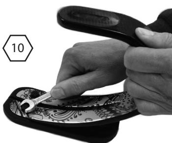
Undo the 2 Heel Spring retaining bolts.
