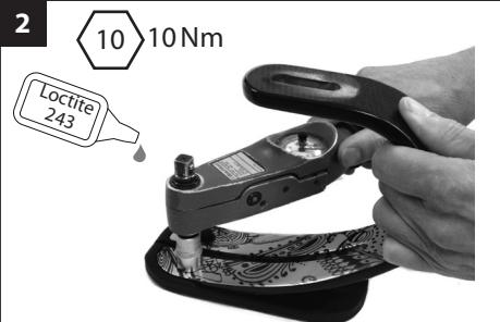
Fit the Toe Spring into the Heel Spring cover and tighten the bolts to 10 Nm.
